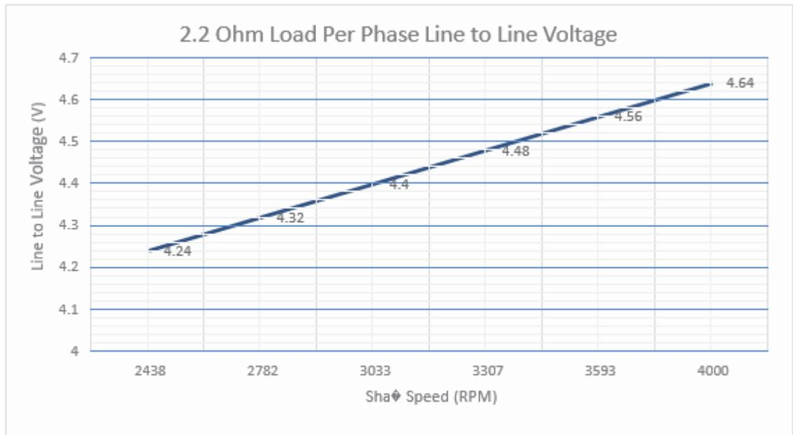
Figure 4: Terminal Voltage with 2.2 Ohm Star-Connected Load
