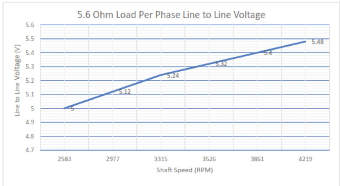
Figure 5: Terminal Voltage with 5.6 Ohm Star Connected Load
