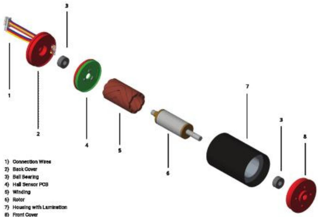
*Figure 7: Manufactured Parts for Small Brushless Coreless Motor (Assun, 2021)*
